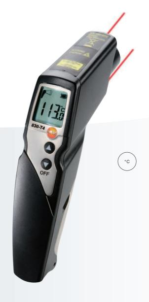
The testo 830 is a universally applicable infrared thermometer for non-contact measurement of surface temperatures in trade and industry. Thanks to a new processor, and therefore better resolution, even more precise measurements are now possible. Temperature can now be recorded to an accuracy of 0.1 °C. Thanks to the min./max. function, the limit values of the last measurement can be displayed and even better monitored.
